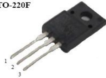
1. Gate 2. Drain 3. Source
