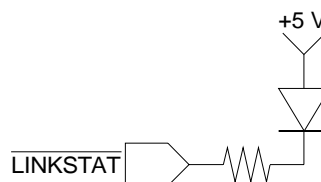
Figure 6. LED Connection Diagram
