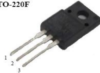
1. Gate 2. Drain 3. Source
