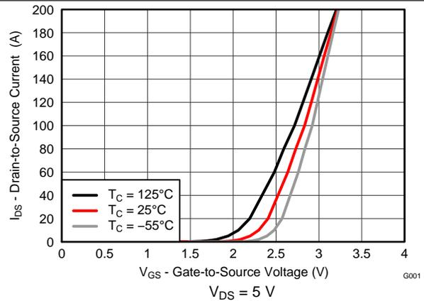
Figure 3. Transfer Characteristics
