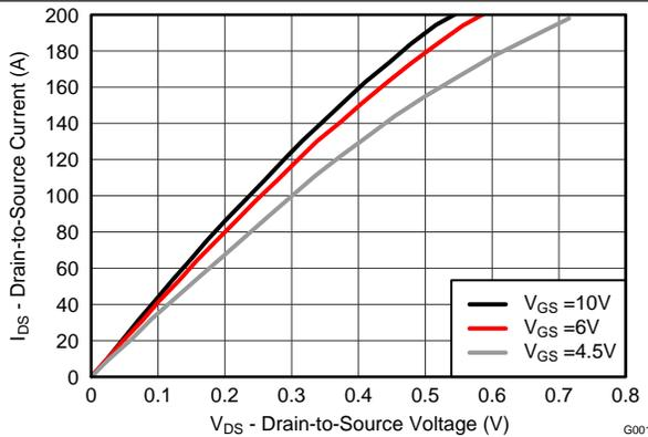
Figure 2. Saturation Characteristics
