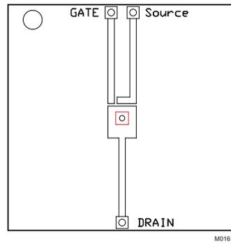
Max  $R_{\theta JA} = 160^{\circ}\text{C/W}$
