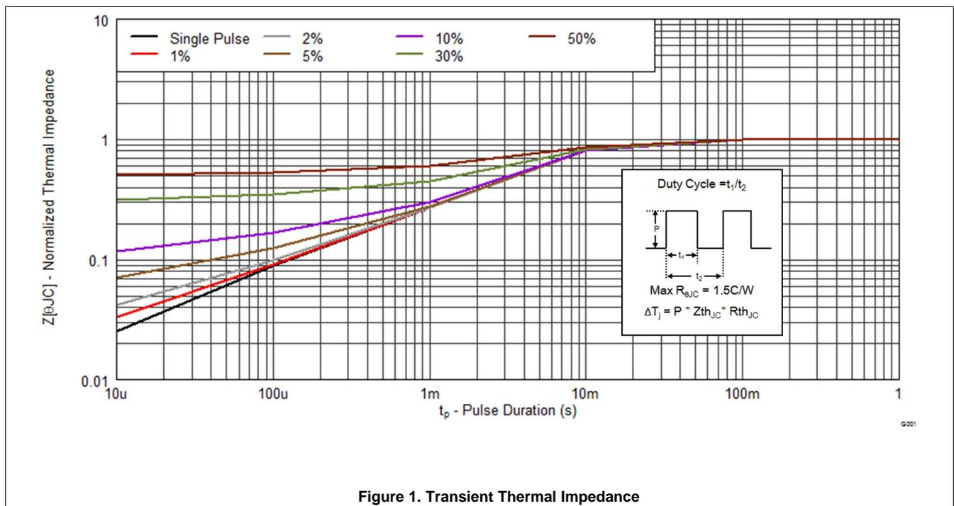
Figure 1. Transient Thermal Impedance
