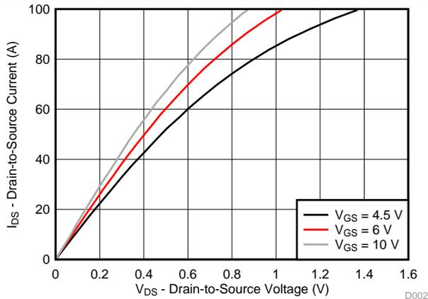
Figure 2. Saturation Characteristics
