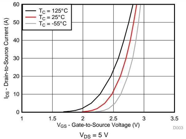
Figure 3. Transfer Characteristics
