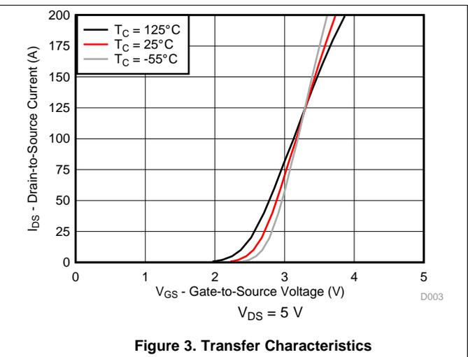
Figure 3. Transfer Characteristics
