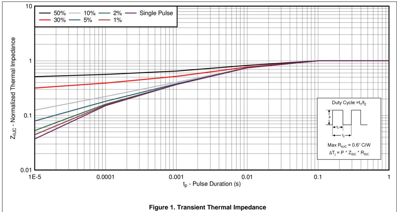
Figure 1. Transient Thermal Impedance
