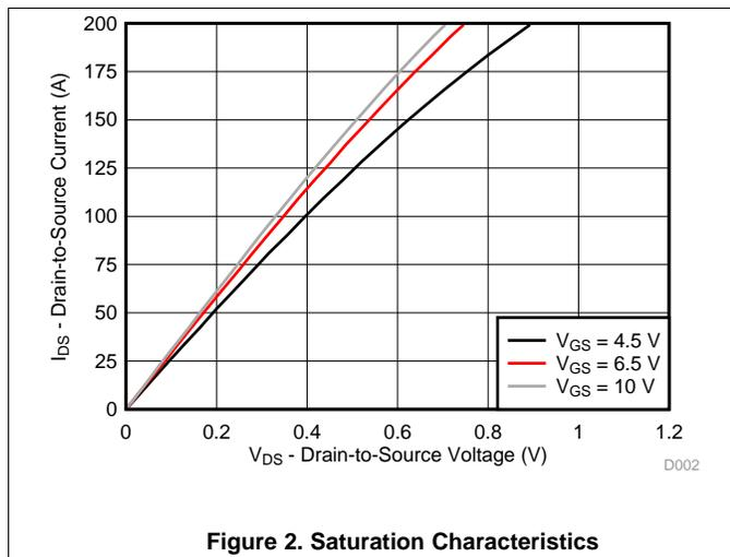
Figure 2. Saturation Characteristics
