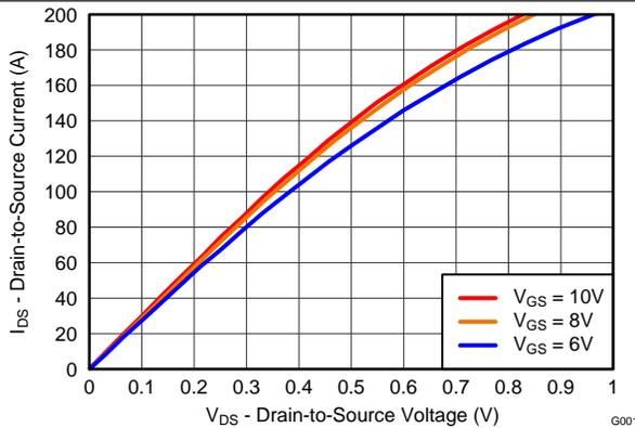
Figure 2. Saturation Characteristics
