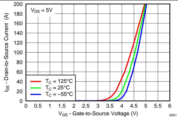
Figure 3. Transfer Characteristics
