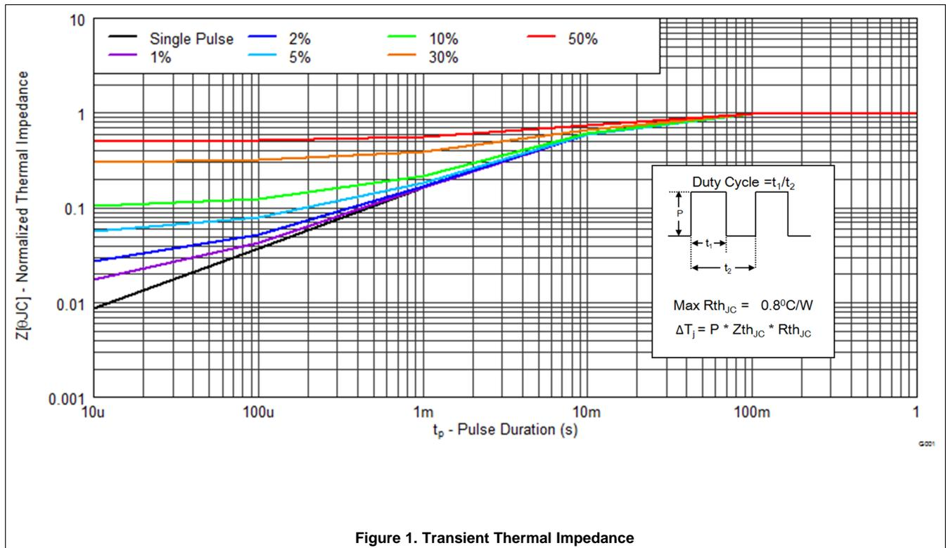
Figure 1. Transient Thermal Impedance
