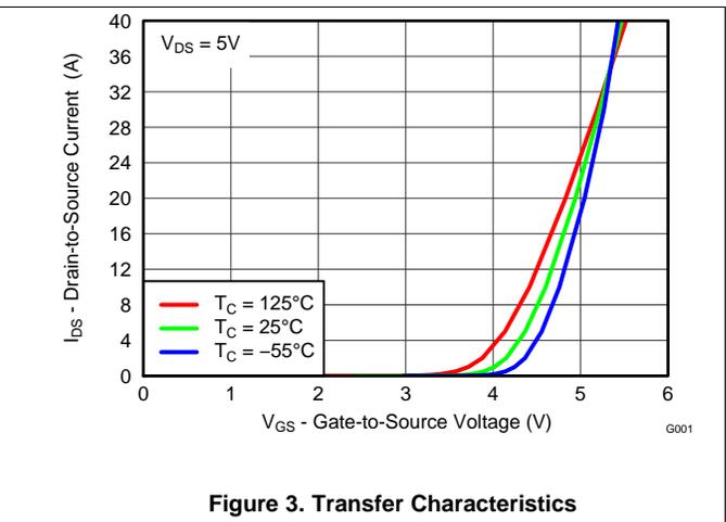
Figure 3. Transfer Characteristics
