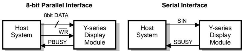
**Monitoring the busy line is recommended, to prevent data loss, and to minimize the delay time for processing subsequent commands / data.**
