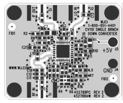
CV110-1A: The application circuit can be broken up into four main functions as denoted in the colored dotted areas above: RF/IF diplexing (purple), amplifier matching (green), filtering (red), and dc biasing (blue). There are various placeholders for chip components in the circuit schematic so that a common PCB can be used for all WJ single-branch converters. Additional placeholders for other optional functions such as filtering are also included.
