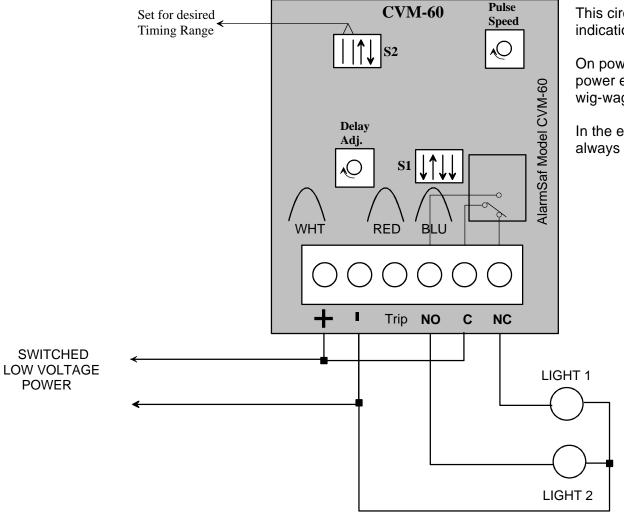
This circuit can be used to provide a unique visual indication for an annuciator or building.
