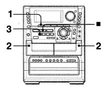
This function allows you to make exact copies of both sides of the original tape. The reverse side of both tapes will start simultaneously as soon as the longer tape has been reversed.
