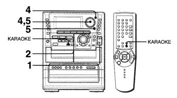
Two microphones (not supplied) can be connected to this unit, allowing you to sing along to music sources. Use microphones with mini plugs ( $\emptyset$ 3.5 mm,  $^{1}/_{8}$  inch).
