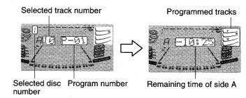
7 Press CD EDIT/CHECK to select side B and program the tracks for side B.
