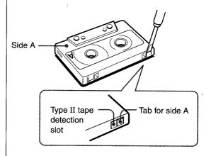
To record on the tape again, cover the tab openings with adhesive tape, etc. (On Type II tapes, take care not to cover the Type II tape detection slot.)
