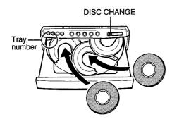
To load three to five discs, press DISC CHANGE to rotate the trays after placing two discs. Place the next disc on the empty tray. Each time DISC CHANGE is pressed, the trays rotate and one disc can be placed.
