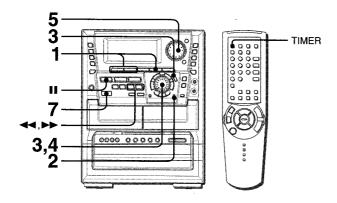
The unit can be turned on at a specified time every day with the built-in timer.
