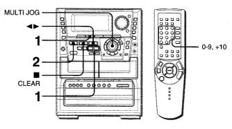
The unit can store a total of 32 preset stations. When a station is stored, a preset number is assigned to the station. Use the preset number to tune in to a preset station directly.
