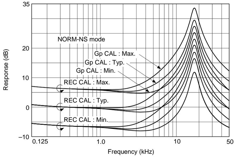
Recording equalizer calibration characteristics (Gp CAL)
