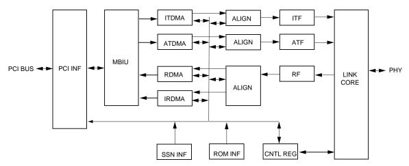
Master Bus Interface MBIU: ITDMA: Isochronous Transmit DMA ATDMA: Asynchronous Transmit DMA
