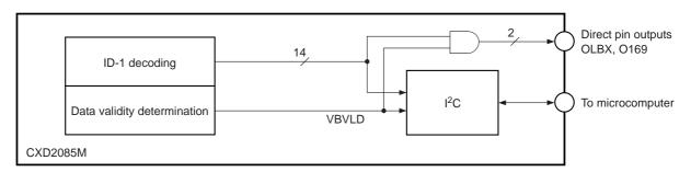
As shown in the figure above, the data validity determination which detects that the valid ID signal is exist or not, and the decoded result are obtained independently during ID-1 decoding. These two results are output to the direct output pins after taking their logical AND.
