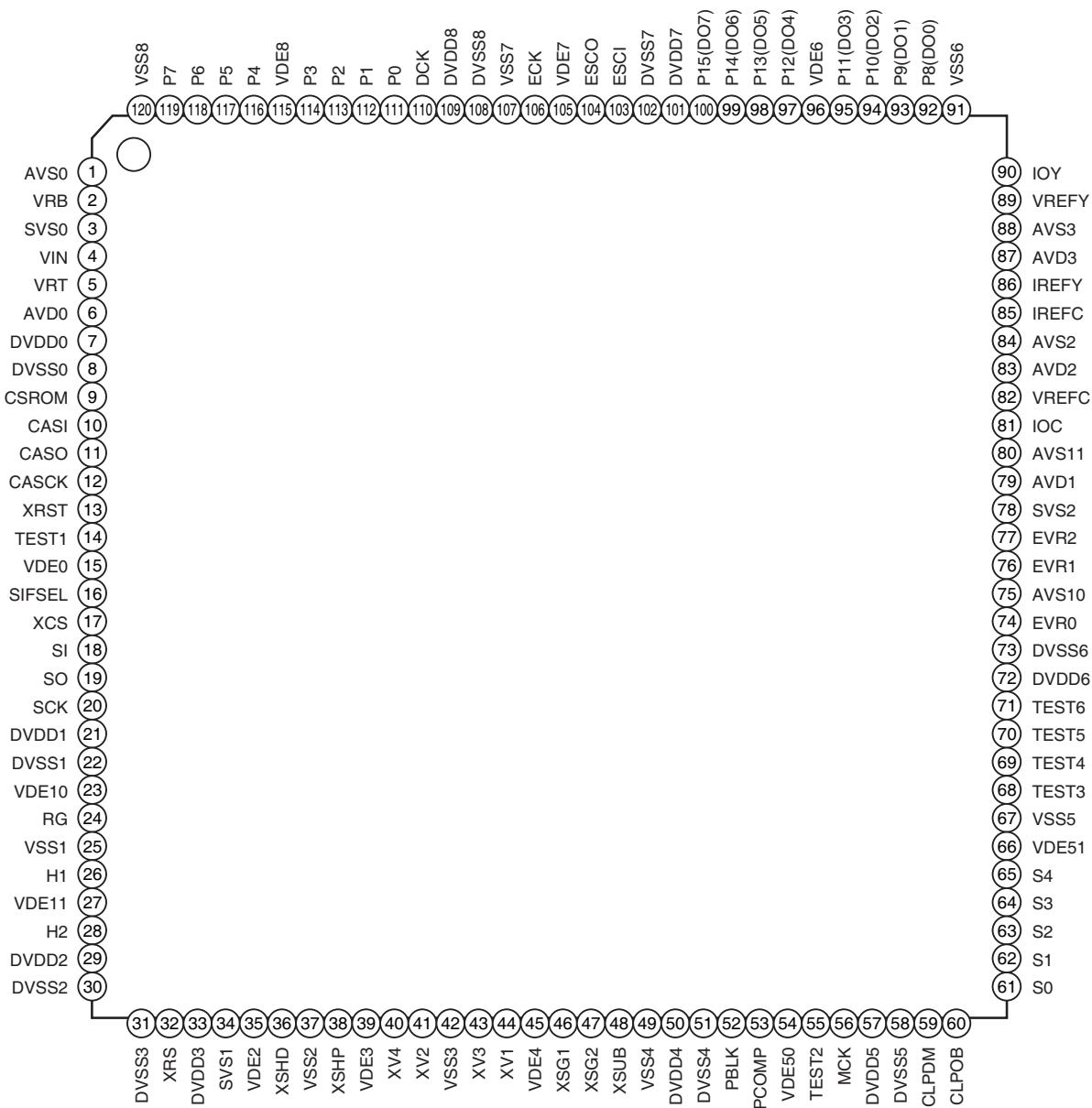
Note) Symbols in parentheses are the signal names when the function is switched by the communication parameter settings.
