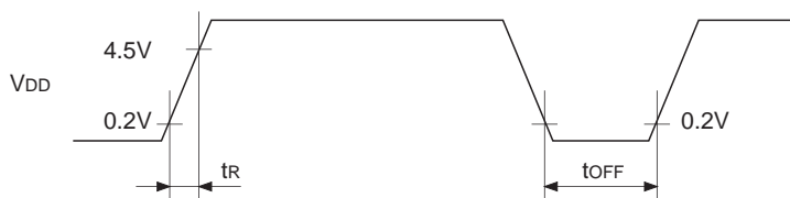
Fig. 11. Power on reset
