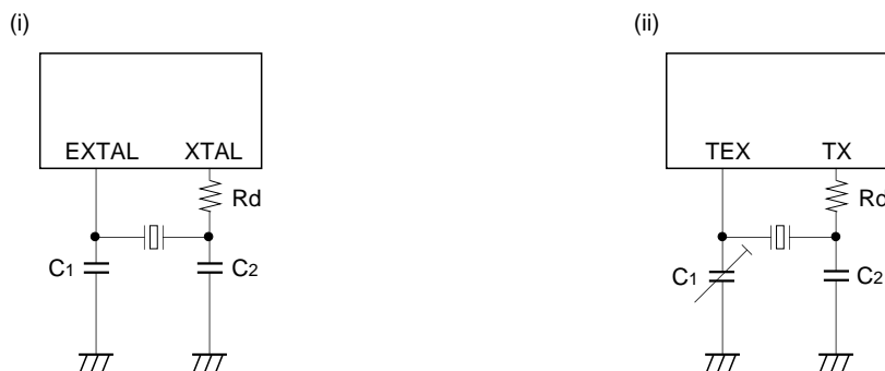
Fig. 10. Recommended oscillation circuit
