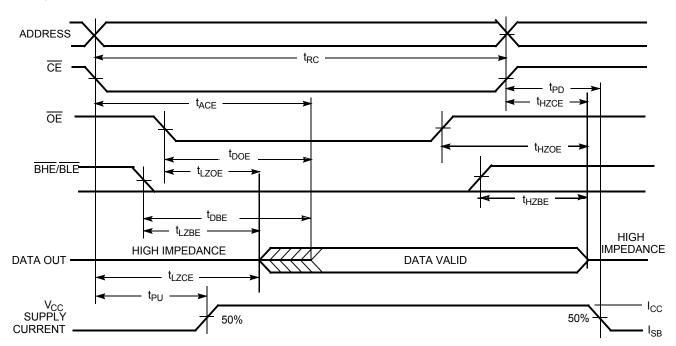
**Notes:** 16. <u>The</u> device is continuously selected.  $\overline{OE}$ ,  $\overline{CE} = V_{IL}$ ,  $\overline{BHE}$  and/or  $\overline{BLE} = V_{IL}$ . 17.  $\overline{WE}$  is HIGH for read cycle. 18. Address valid prior to or coincident with  $\overline{CE}$  and  $\overline{BHE}$ ,  $\overline{BLE}$  transition LOW.
