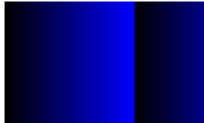
Pattern 13: 256 blue grayscale / two pixels From 0 to 255
