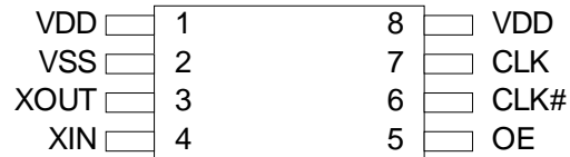
Figure 1. 8-pin TSSOP pinout
