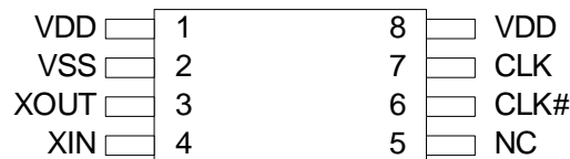
Figure 1. Pin Diagram - 8-Pin TSSOP
