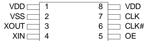
Figure 1. 8-pin TSSOP pinout
