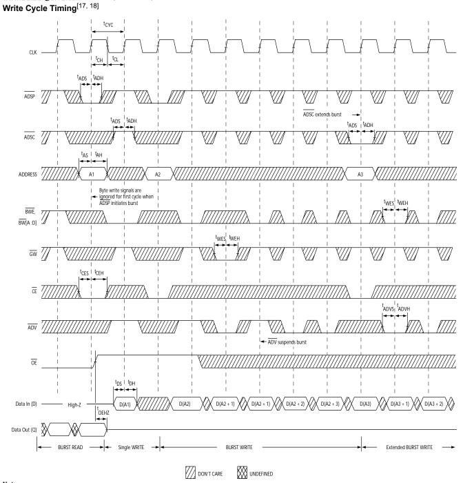
**Note:** 18. Full width Write can be initiated by either  $\overline{GW}$  LOW; or by  $\overline{GW}$  HIGH,  $\overline{BWE}$  LOW and  $\overline{BW}_{[A:B]}$  LOW.
