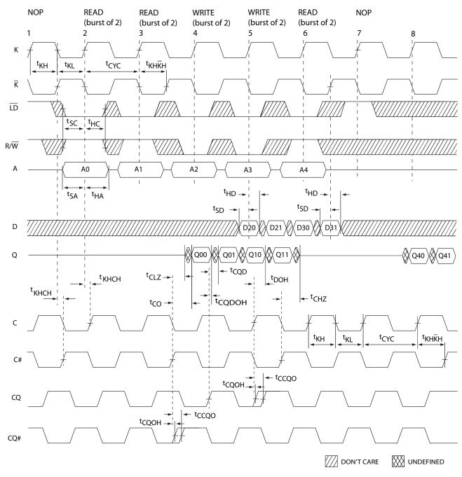
29. Q00 refers to output from address A0. Q01 refers to output from the next internal burst address following A0, i.e., A0+1.
