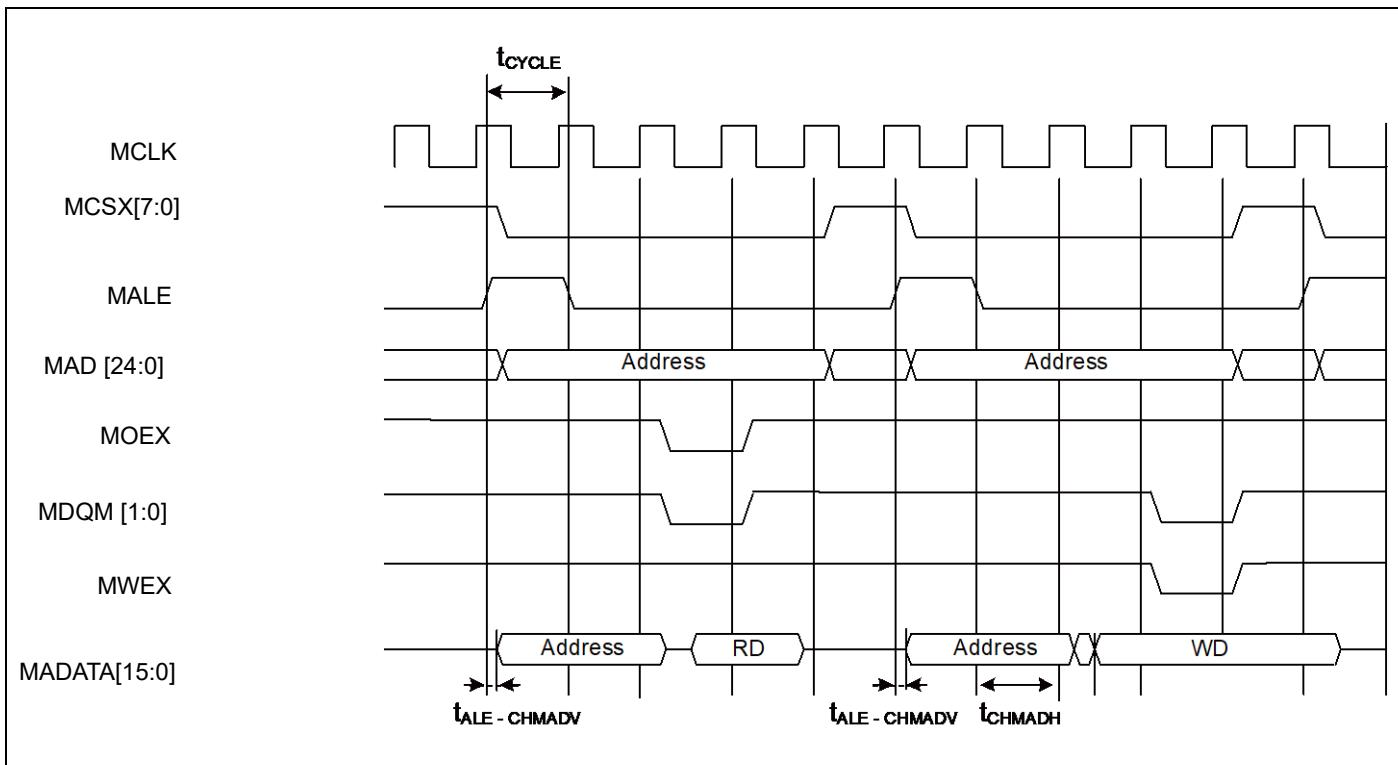
**Multiplexed Bus Access Synchronous SRAM Mode**
