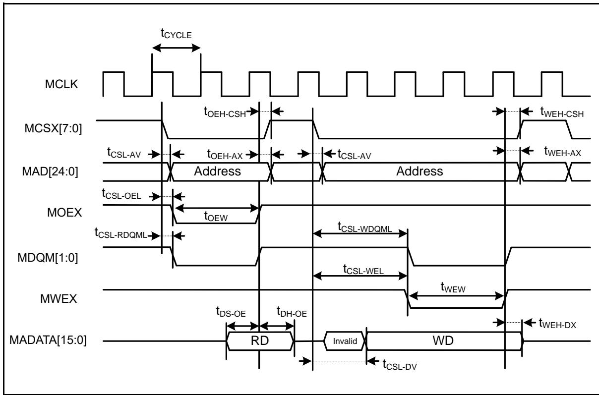
**Separate Bus Access Synchronous SRAM Mode**
