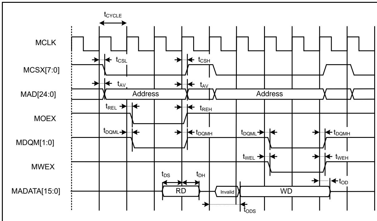
**Multiplexed Bus Access Asynchronous SRAM Mode**
