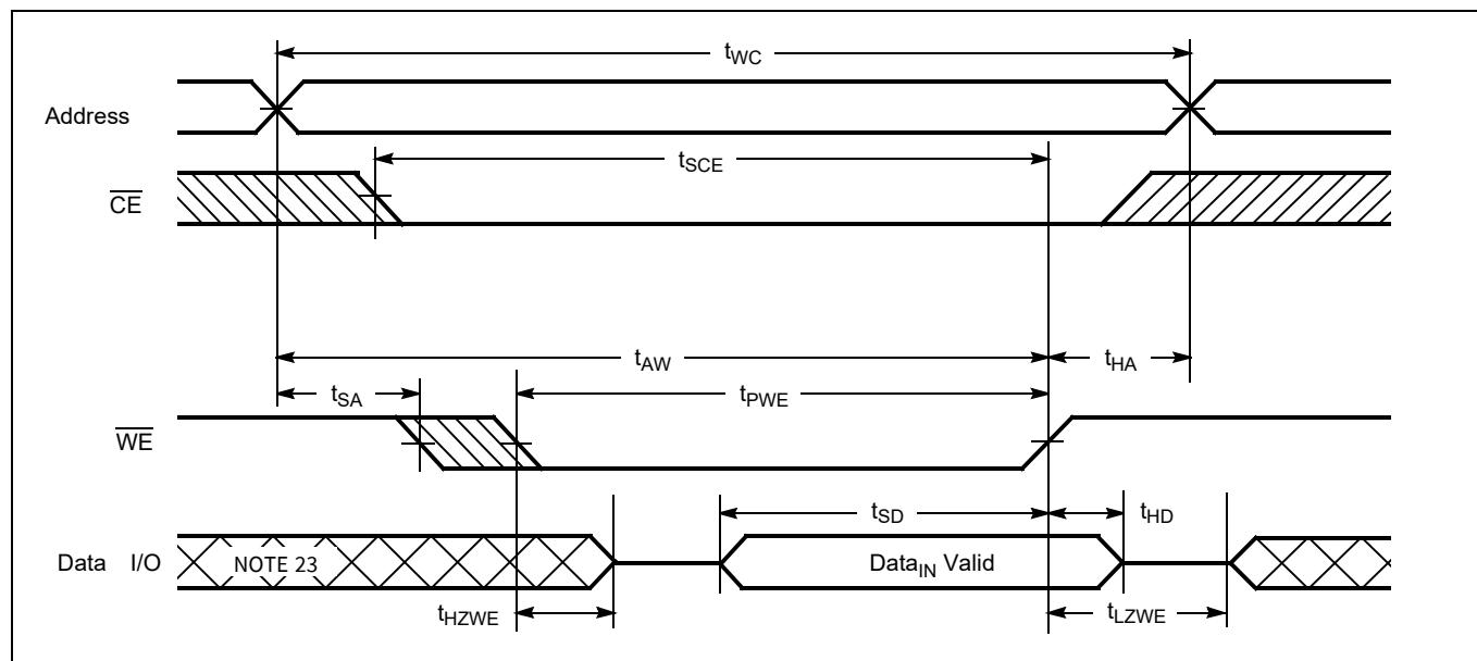
Figure 8 Write cycle No. 3 ( $\overline{WE}$  Controlled,  $\overline{OE}$  LOW)**Note**
