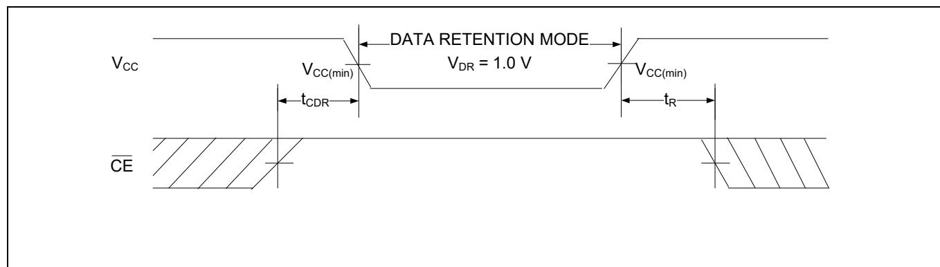
**Figure 3 Data retention waveform**
