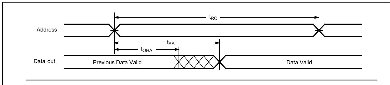
Figure 4 Read cycle No. 1<sup>[16, 17]</sup>
