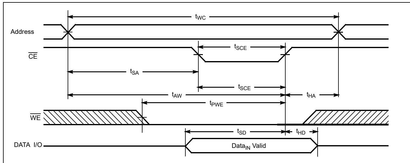
Figure 6 Write cycle No. 1 ( $\overline{CE}$  Controlled)<sup>[20, 21]</sup>
