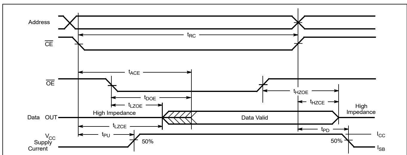
Figure 5 Read cycle No. 2 ( $\overline{OE}$  Controlled,  $\overline{WE}$  HIGH)<sup>[18, 19]</sup>
