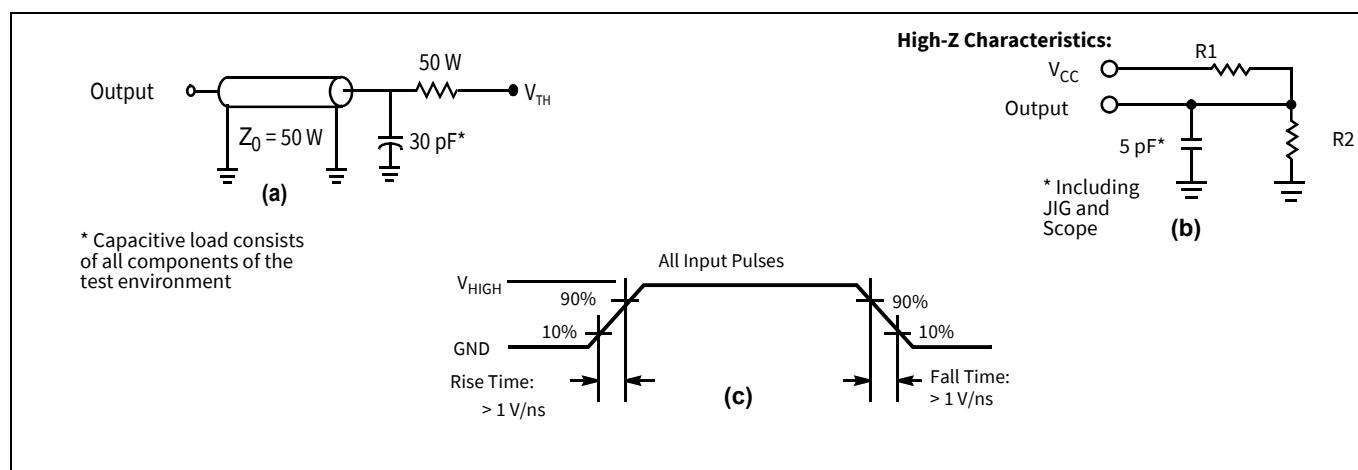
Figure 2 AC test loads and waveforms<sup>[7]</sup>
