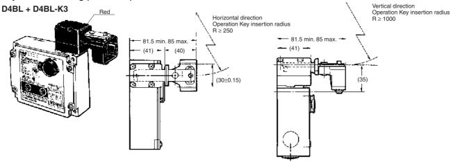
Note: 1. Unless otherwise specified, a tolerance of  $\pm 0.4$  mm applies to all dimensions.
