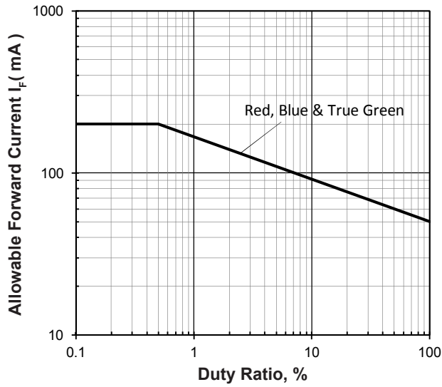
Allowable Forward Current Vs Duty Ratio ( T_j = 25^\circ\text{C} ; t_p \leq 10\mu\text{s} )
