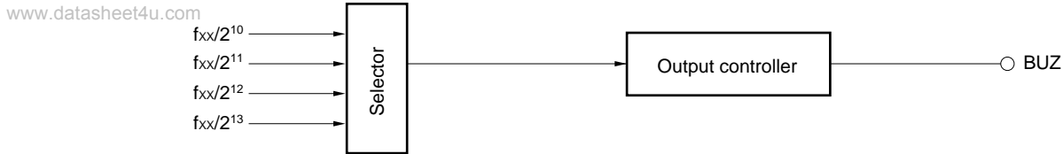
Figure 7-15. Block Diagram of Buzzer Output Function
