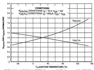
TYPICAL NORMALIZED  $R_{DS(ON)}$  AND  $V_{GS(TH)}VS$ . TEMP.
