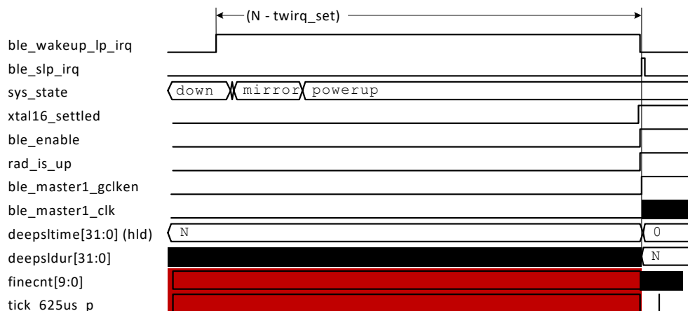
Figure 119: Exit BLE Deep Sleep Mode at predetermined time (zoom out)
