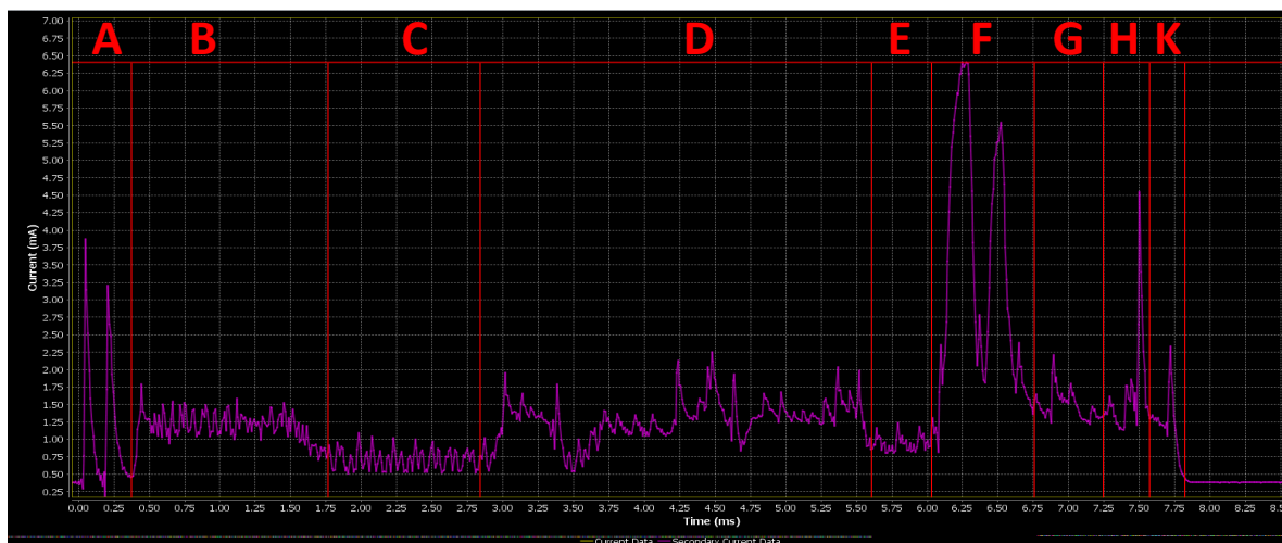
Figure 129: BLE Connection power profile
