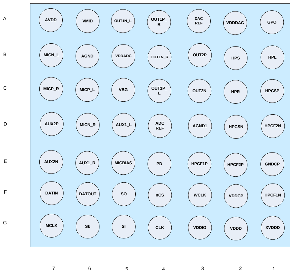
Figure 2: DA7210 pad arrangement (bottom view ball side up)
