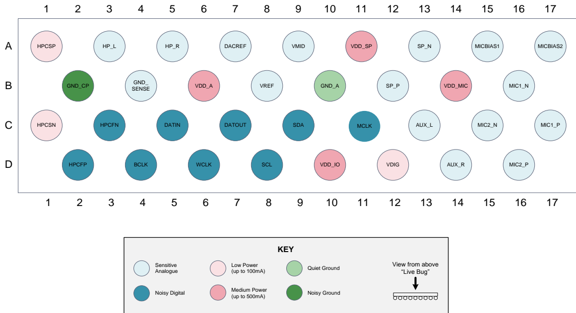
Figure 3: DA7212 ball layout
