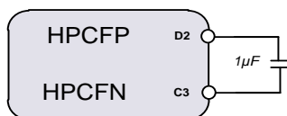
Figure 39: Charge Pump Flying Capacitor
