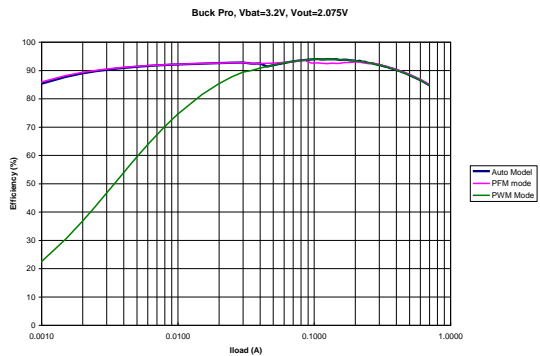
Figure 10: BUCKPRO efficiency curves
