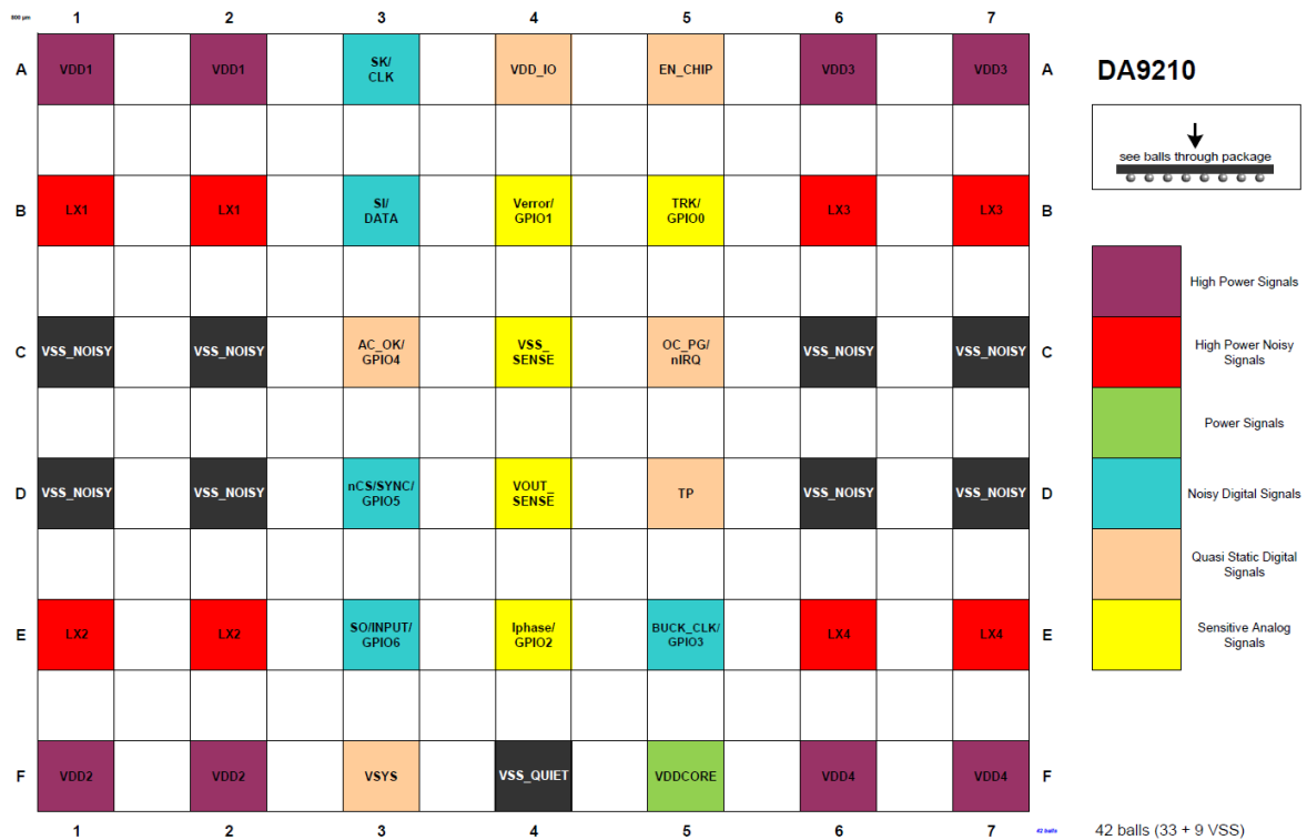
Figure 3: Connection Diagram (42 VFBGA)
