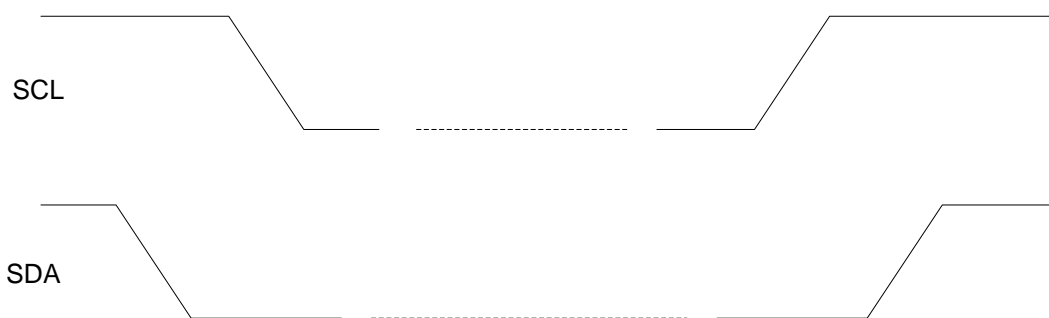
Figure 22: Timing of 2-WIRE START and STOP Condition
