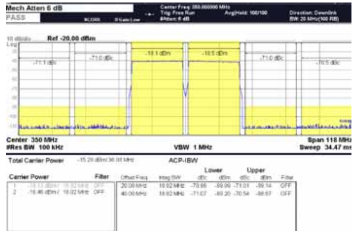
Fig 22. ACLR of 2 carriers LTE (BW=2 x 20 MHz) centered at 350 MHz
