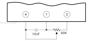
Adjust/comp (pin 4) may be driven by external circuitry referenced to pin 2 (-output) if desired. Grounding pin 4 causes voltage to increase (25% typically) while driving pin 4 above 1.3V causes output voltage to decrease. Pin 4 may be driven negative without damage, however the resultant increase in converter output voltage should be considered. Pin 4 may be driven through  $10 \mathrm{K}\Omega$  or more if connection of the comp function is also required.
