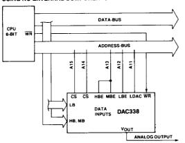
This mode of operation requires 13k bytes of unused addresses. No additional address decoder is necessary. The two chip-select inputs together with the byte-enable and load-DAC inputs are used to control all functions of the DAC. Through selecting the addressines the user can vary the addresses used to control the DAC. In the above figure the control signals have the following address-configurations (hex):
