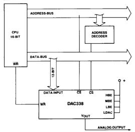
Interfacing the DAC338 to a 16-Bit microprocessor is quite easy, because no multiplexing of the data inputs is necessary. An address decoder and the second chip-select input is used to select the DAC.
