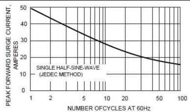
FIG. 1 FORWARD URRENT DERATING CURVE
