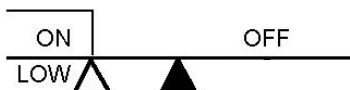
Figure 4-5 Lower Limit Deviation Alarm (Alarm Code 12, No alarm release in the first alarming situation)
