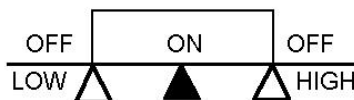
Figure 4-8 Deviation Band Alarm [Hold On = Yes] (Alarm Code 04, Alarm release in the first alarming situation)
