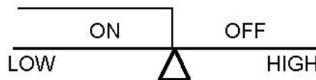
Figure 4-14 Absolute Lower Limit Alarm (Alarm Code 16, No alarm release in the first alarming situation)
