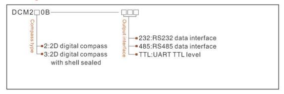
E.g: DCM220B-232: 2D without enclosure sealed /RS232 output
