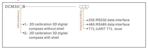
E.g: DCM302B-232: Plane calibration 3D electronic compass(with enclosure sealed)/RS232 output
