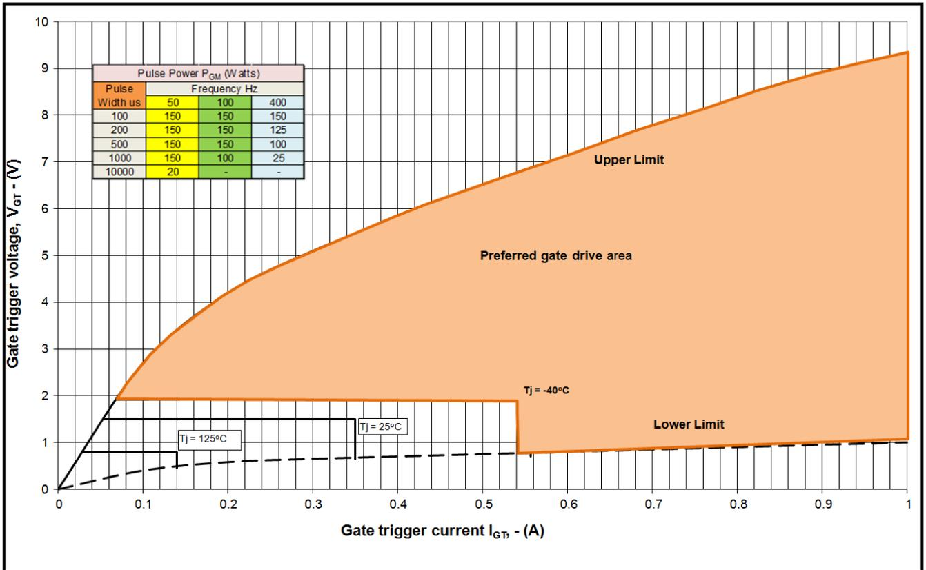
Fig14 Gate Characteristics
