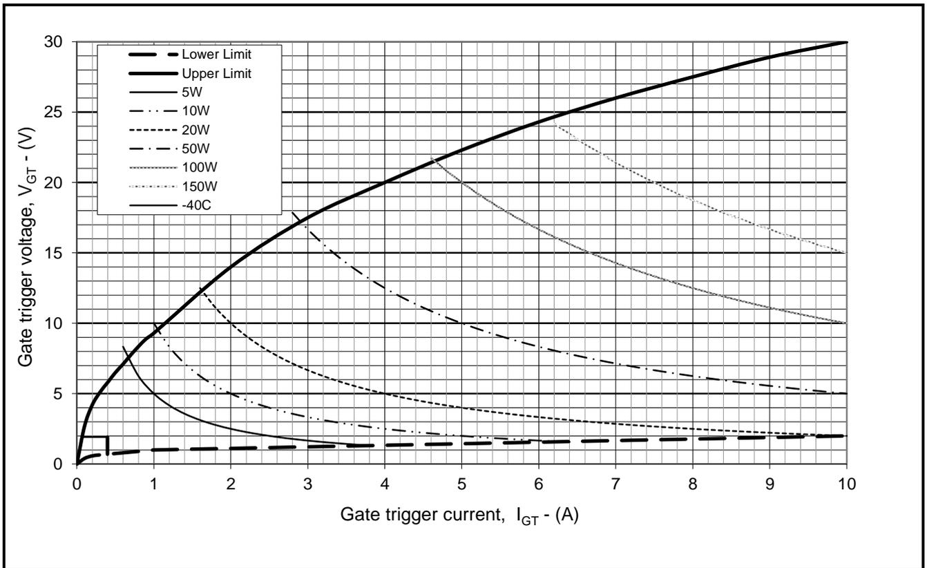
Fig. 15 Gate characteristics
