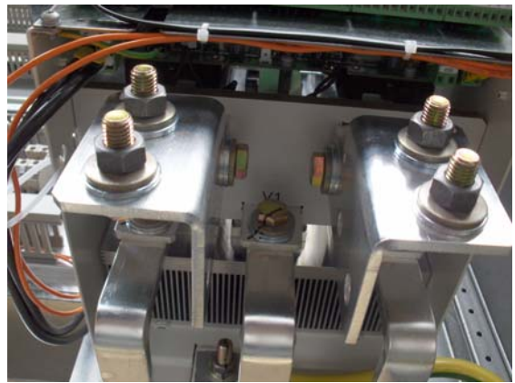
Bottom view of lug bar mounted on a D4 module
