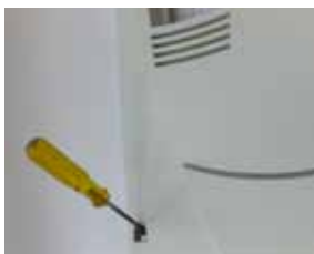
Remove the DCS800 Control Panel if present. Depress the locks to remove the cover
