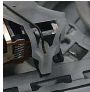
[Incorrect built-in state] The chassis is not nipped between the PU case and the PU rack.
